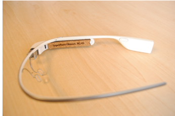
Figure 2: Headset with heatshield design informed by study participants. The “SuperpowerGlass” name was adopted from a child’s description that the system’s prediction of emotions made them feel as if they had superpowers.
