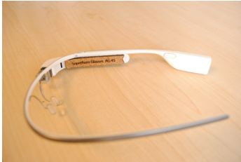
Figure 2: Headset with heatshield design informed by study participants. The “SuperpowerGlasses” name was adopted from a child’s description that the system’s prediction of emotions made them feel as if they had superpowers.
